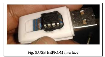
EEPROM interface is provided such that it uses the same address in both programmer and the M4 driving card. The device address used is 0x50. In programmer, it is required to transfer data fast so we use page transfer of data, which takes 1–2 seconds to transfer all data in the EEPROM. While in driving card M4 module is operated according to each byte of EEPROM with speed information given by sensor, so we read data byte by byte.
