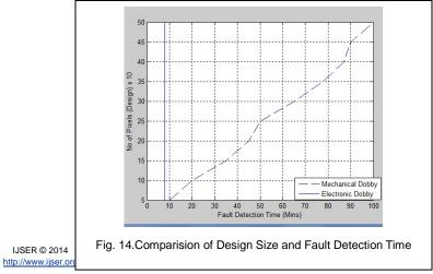
The above graph shows fault detection time versus No. of pixels characteristics. Fault detection is very difficult in mechanical system as increasing number of pixels will increase length of punching card chain. If we are using 400 punching cards, then we will have to check all these cards. While in electronic system, it is quite handy to replace any faulty pattern. Fault detection and replacement of faulty part will not take more than 10 minutes time.
