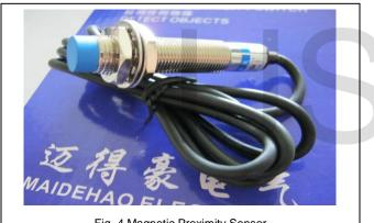
Fig. 4.Magnetic Proximity Sensor
