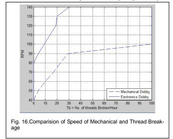
The graph above depicts number of threads breakage versus speed characteristics. It can be observed that in electronic system, no thread is broken until the speed of 80 rpm of the machine. But with the mechanical system thread breakage is too much at 80 rpm. It has an increasing trend at higher speed but
